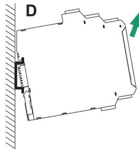
D. Remove the apparatus as arrow shows.
